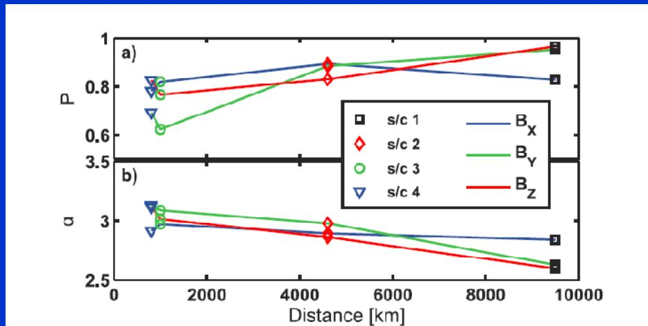
FIG. 4 (color). Intermittency parameter  $P$  (panel a) and spectral slope  $\alpha$  (panel b) as functions of the BS distance. The colors represent the magnetic field components— $B_X$  (blue),  $B_Y$  (green), and  $B_Z$  (red), with the spacecraft symbol in color for each  $P$  estimation.
